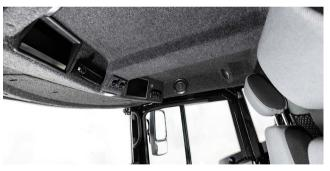
A long roof protects the user from direct sunlight regardless of the large window areas. User comfort is further boosted by bottle storage with cooling and heating, in-cabin smartphone charging and plenty of storage space for documents and tools.
