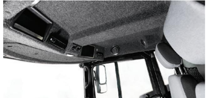
A long roof protects the user from direct sunlight regardless of the large window areas. User comfort is further boosted by bottle storage, in-cabin smartphone charging and plenty of storage space for documents and tools.
