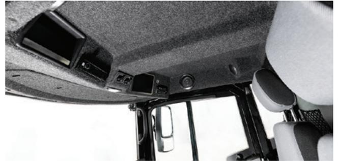
A long roof protects the user from direct sunlight regardless of the large window areas. User comfort is further boosted by bottle storage with cooling and heating, in-cabin smartphone charging and plenty of storage space for documents and tools.
